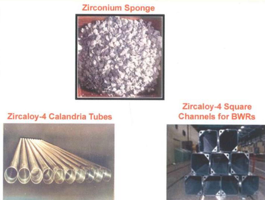
Fig. 7.2 Zirconium sponge and zircaloy products.
